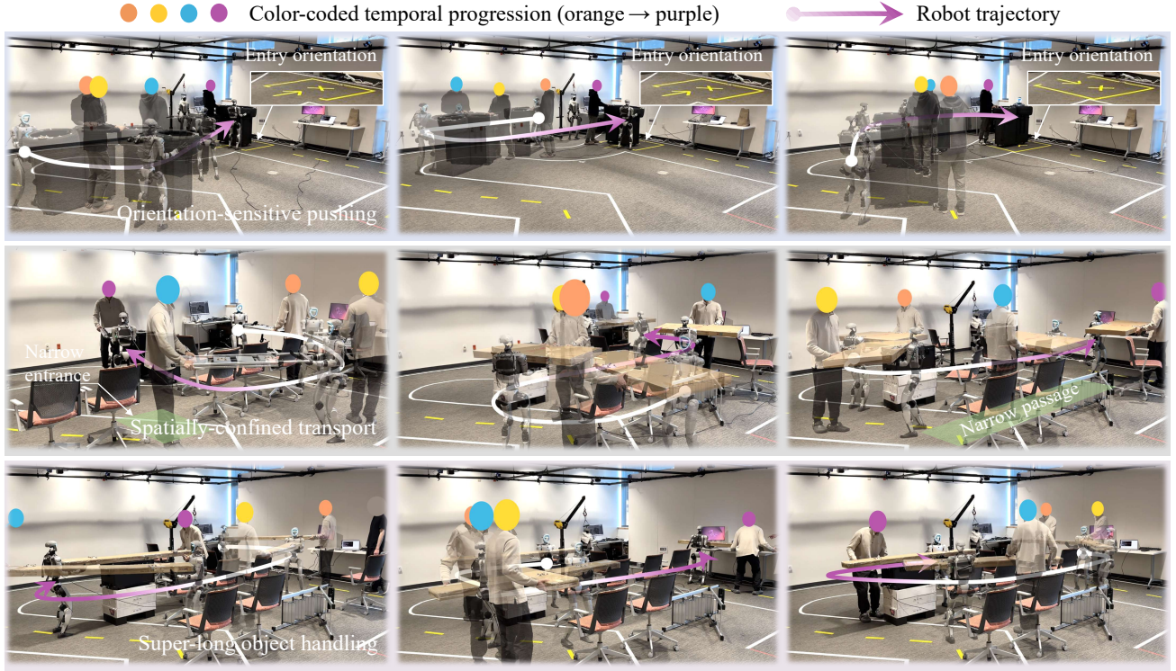
Figure 8. Sim-to-real deployment across embodied tasks: macro-view of deployment on OSP (top), SCT (Middle) and SLH (Bottom). Temporal progression is indicated by color gradients; arrows trace the stable trajectories maintained by HALO despite complex physical coupling and human-induced perturbations.
